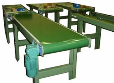
Fig.3 Short horizontal conveyor with the PVC belt, [4]
