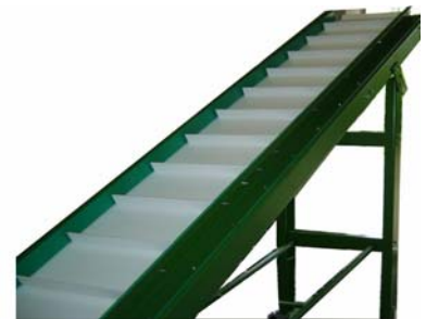
Fig.4 Inclined up conveyor with the ribbed PVC belt, [4]
