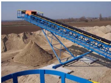
Fig.2 Typical belt conveyor for transport of bulk solids, [3]
